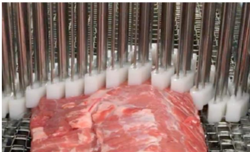
Figure 1.2: Precision Injection System in Meat Processing (Philipsen and Moeslund, 2019)
