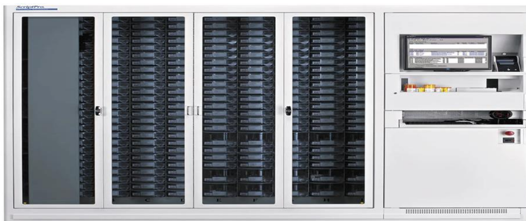
Figure 2: MEDICINE AUTOMATED DISPENSING SYSTEM CRS 225 (ScriptPro, 2024b): Channel-fed dispensing systems store drugs in individual metal or plastic channels, with each channel
