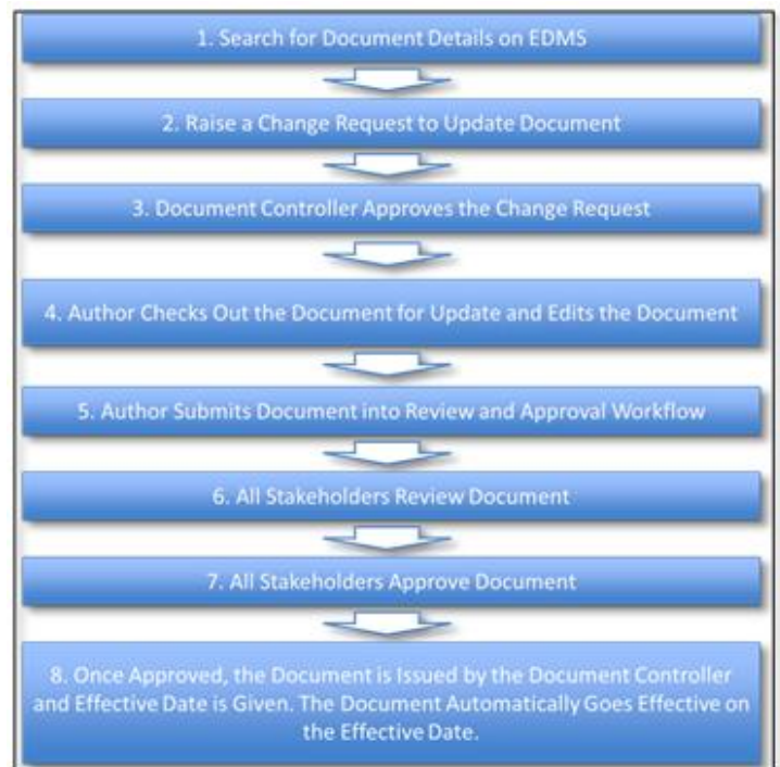
Figure 8 Process mapping of Electronic Document Management System
