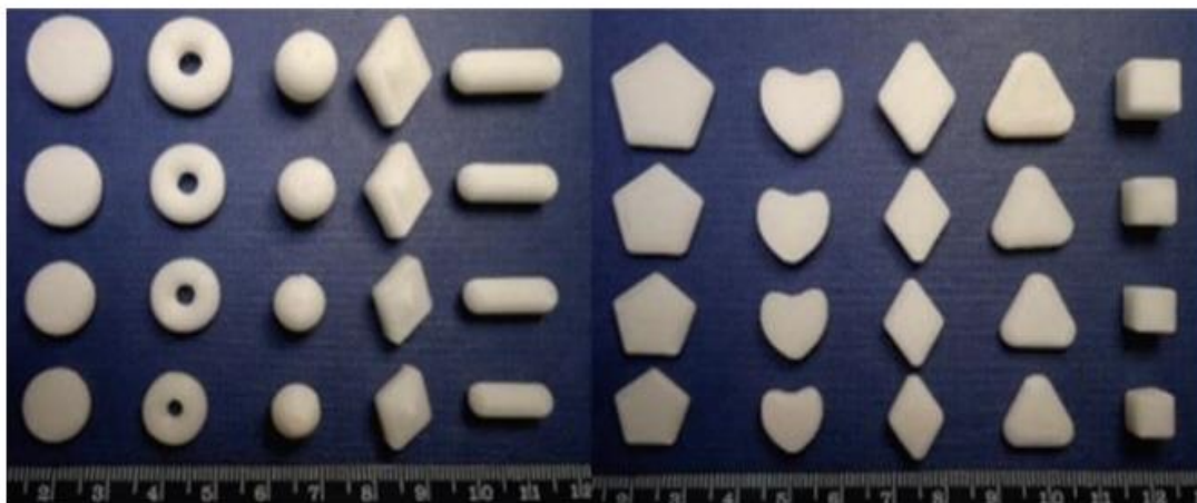
Figure 9. Range of shapes and sizes of 3D printed tablets (Trenfield et al., 2018, P. 8)
