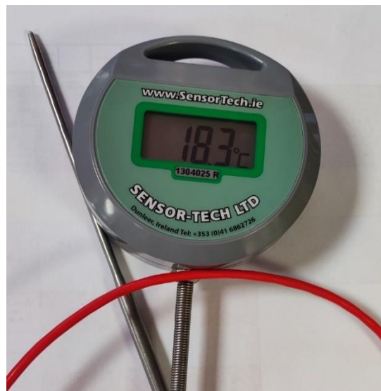
Image 3.3.1 Temperature probe (Sensor Tech LTD), taken during the cooking procedure in NPD kitchen 2023.
